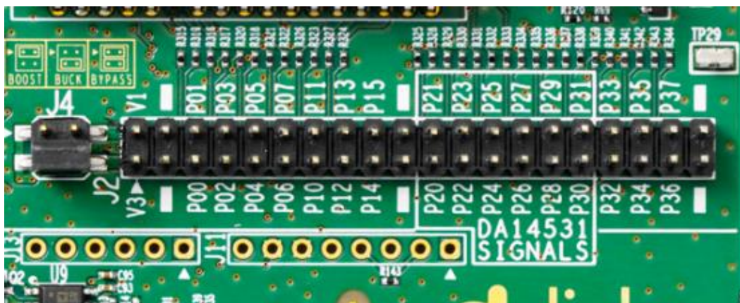
Figure 18: J2, Breakout Header of DA14531 PRO-MB
