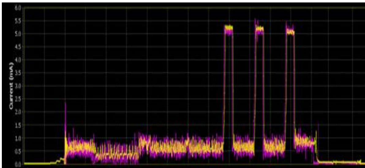
Figure 37: Current Measurement Presented in Power Profiler of SmartSnippets Toolbox
