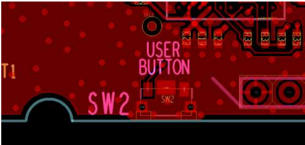
Figure 15: General Purpose Push Button SW2
