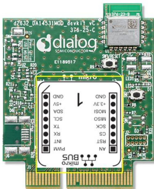
Figure 18: Example of mounting MikroBUS™ module
