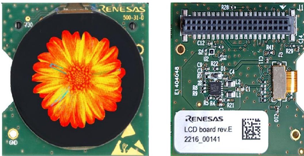
Figure 48: LCD TFT Daughterboard Top (Left) and PCBA Bottom Side (Right)
