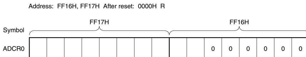
Figure 12-2. Format of A/D Conversion Result Register 0 (ADCR0)
