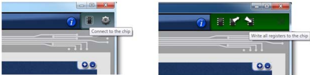
Figure 3. Connecting to the chip: Left: click on the chip symbol to make the connection; Right: A green area appears if I 2 C communication is established.
