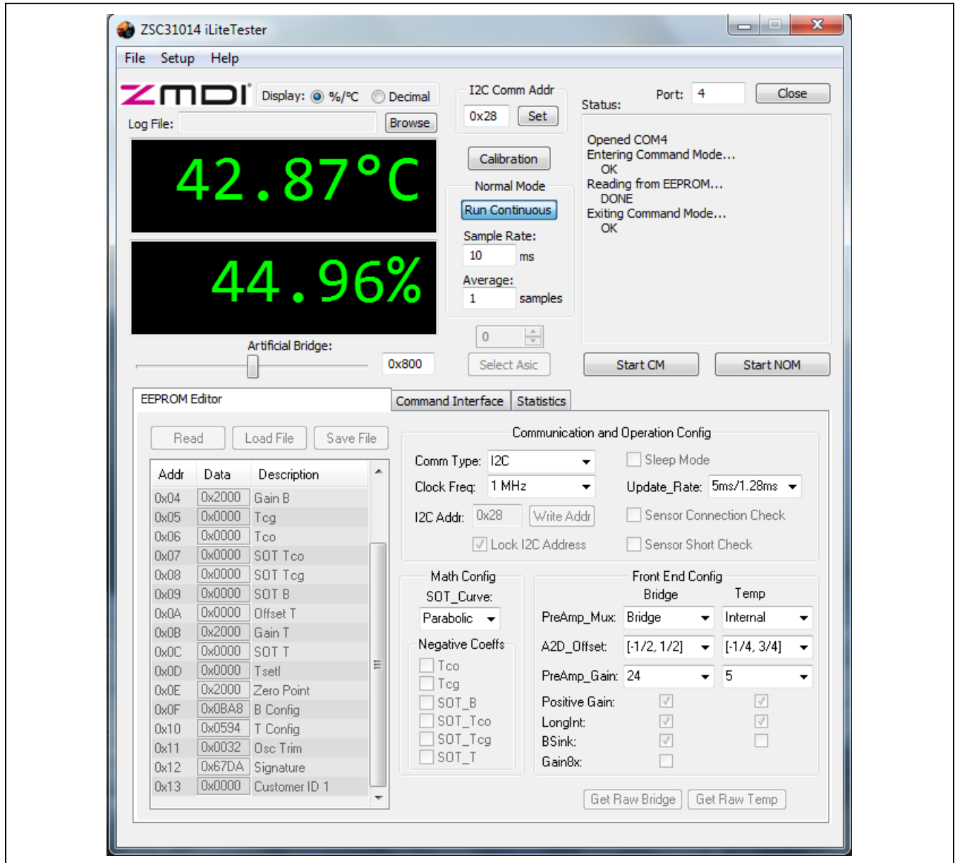
Figure 4.1 Bridge and Temperature Measurements Display
