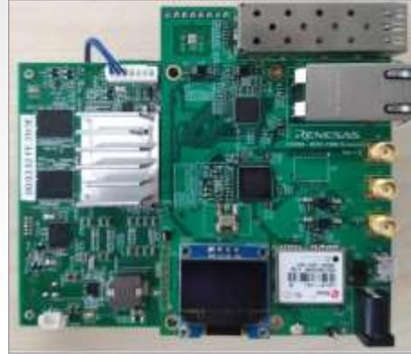
CN268 IEEE-1588 Solution for Synchronization of timing networks
