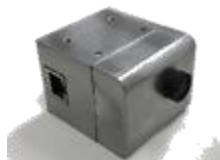
PoE camera module w/ RZ/V2M
