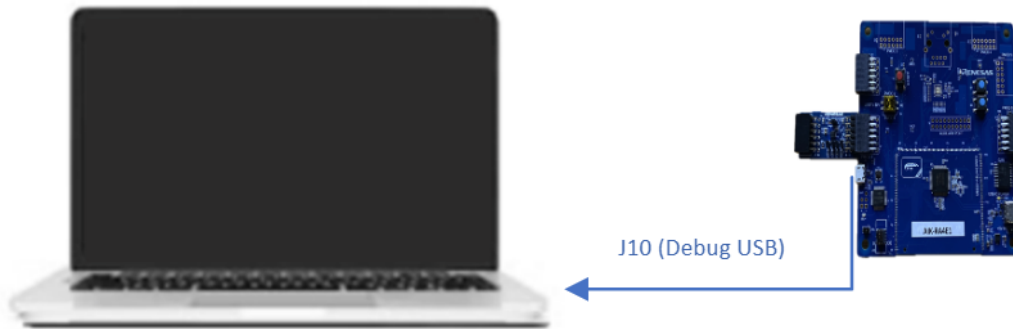
Figure 16. Connecting the AIK-RA4E1 Board to the Host PC via USB Debug Port
