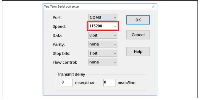
Figure 9. Select 115200 on the Speed Pulldown
