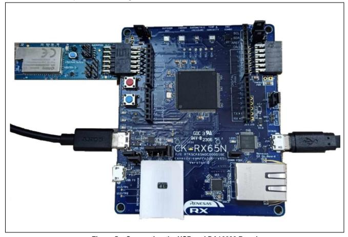
Figure 5. Connecting the USB and DA16600 Pmod
