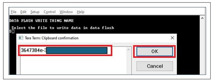
Figure 42. Storing the Thing Name into the Data Flash
