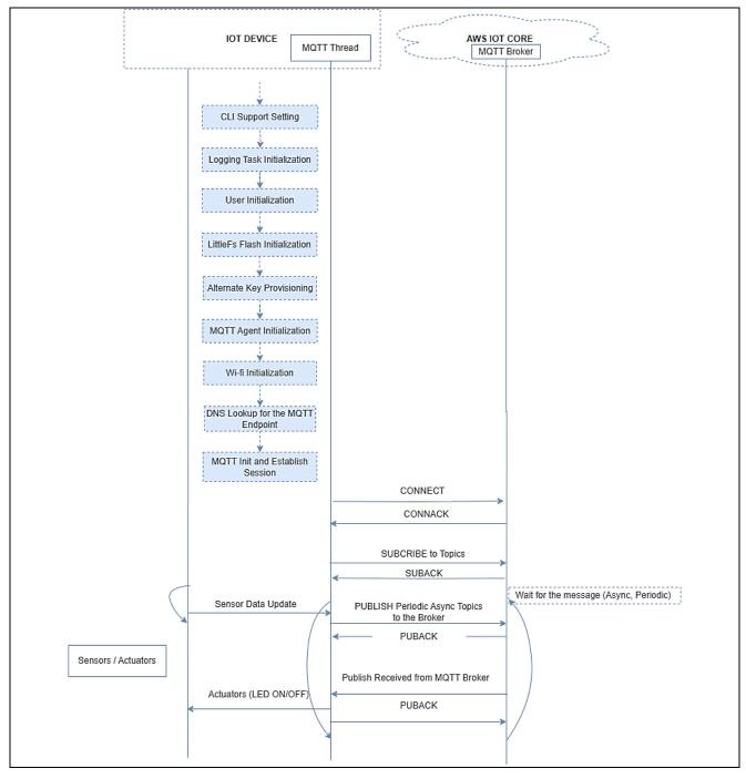
Figure 4. Application Example Implementation Details
