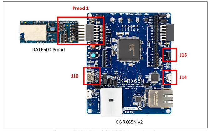
Figure 1. CK-RX65N v2 (with Wi-Fi DA16600 Pmod)
