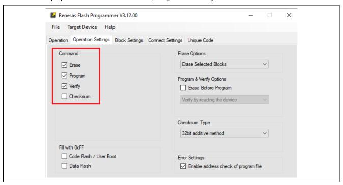
Figure 122. Flash the Firmware (1/3)
