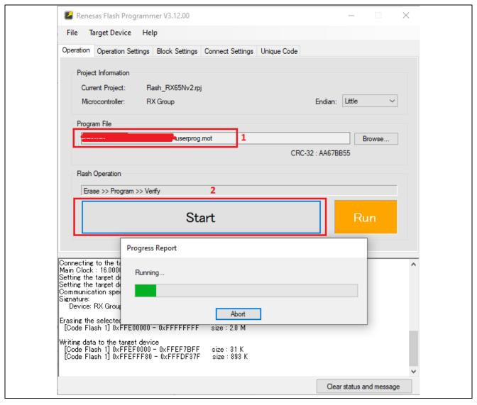
Figure 123. Flash the Firmware (2/3)
