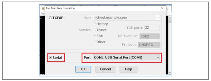
Figure 7. Selecting the Serial Port on Tera Term
