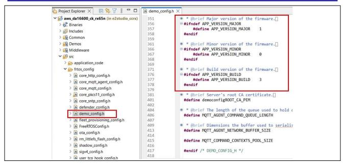
Figure 132. Setting New Version for Firmware
