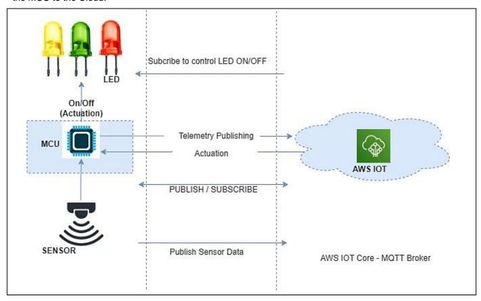
Figure 3. MQTT Publish/Subscribe to/from AWS IoT Core
