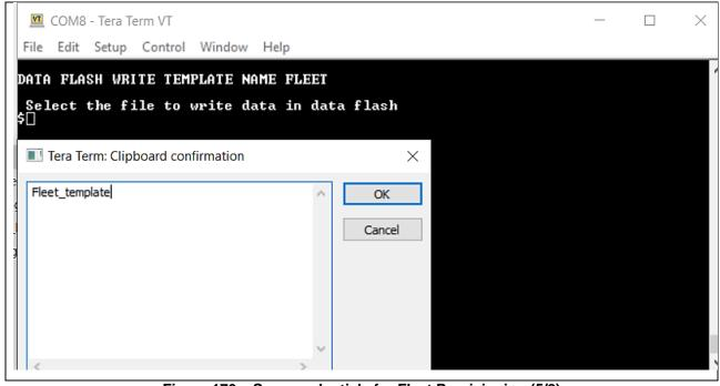
Figure 170. Save credentials for Fleet Provisioning (5/8)
