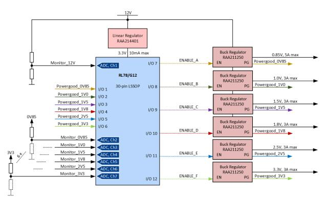
Fig.1 Flexible 6-Channels Power Sequencer block diagram
