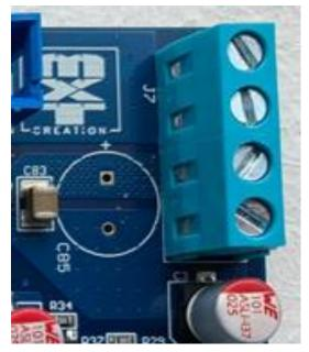
Fig.4 Electrolytic capacitor position
