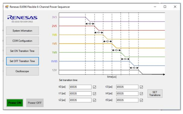
Fig.10 GUI – Set OFF Transition Time menu
