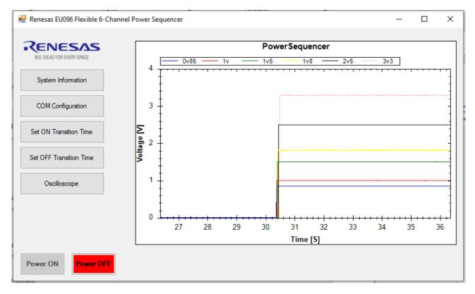
Fig.11 GUI – Oscilloscope menu
