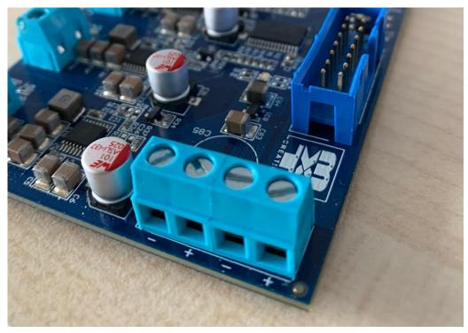
Fig.6 Flexible 6-Channels Power Sequencer screw terminal
