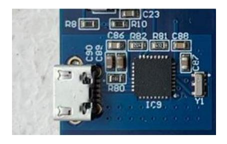
Fig.8 Flexible 6-Channels Power Sequencer micro-USB connector
