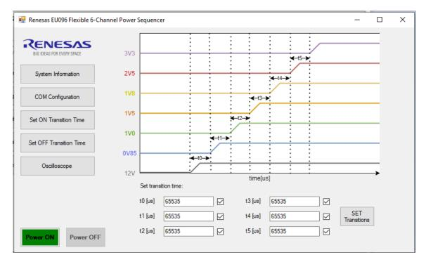
Fig.9 GUI – Set ON Transition Time menu
