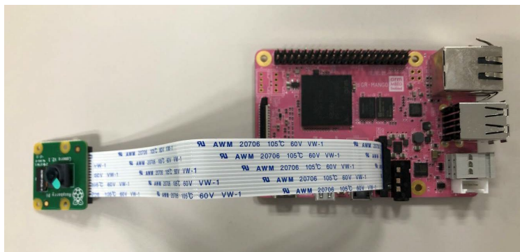
Figure 6-22 Connecting target board and MIPI Camera
