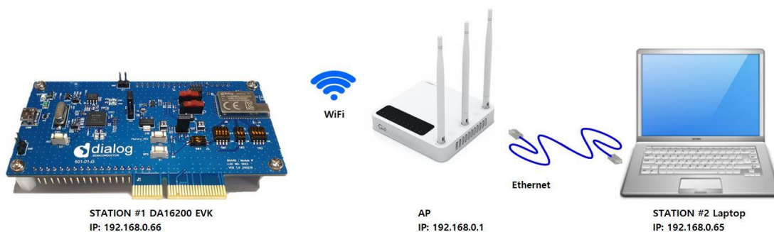
Figure 46: Ping Test Environment
