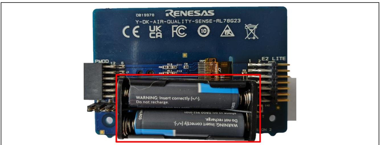
Figure 4. Batteries
