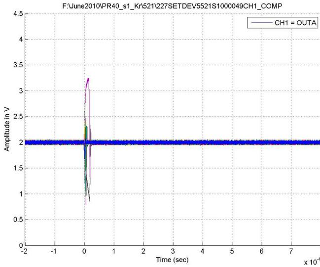
Figure 21. Typical Capture at  $V_S = \pm 4.5V$ , Channel A, LET = 28MeV·cm<sup>2</sup>/mg, Run 521
