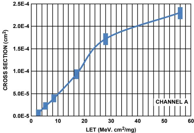
Figure 5. Channel A SET Cross Section vs LET for  $V_S = \pm 18V$  with 90% Confidence Level Interval Bars
