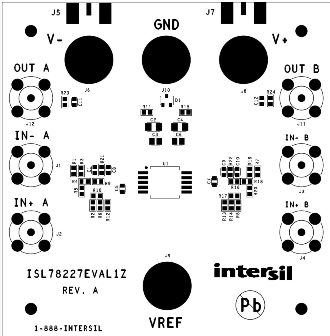
Figure 30. ISL70227SxH SEE Test Board Top View
