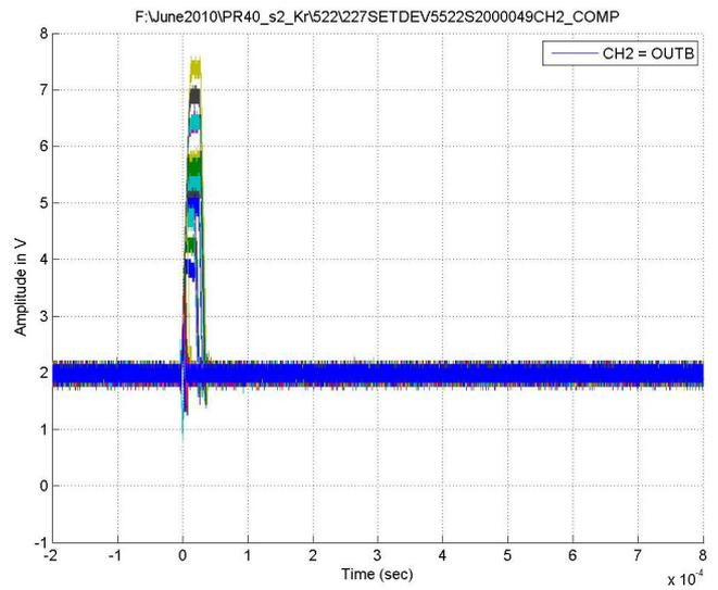
Figure 24. Typical Capture at  $V_S = \pm 18V$ , Channel B, LET = 28MeV·cm<sup>2</sup>/mg, Run 512
