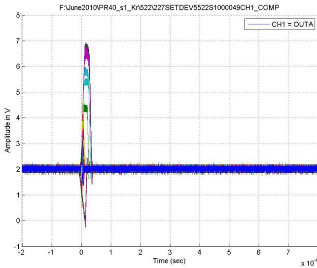
Figure 23. Typical Capture at  $V_S = \pm 18V$ , Channel A, LET = 28MeV·cm<sup>2</sup>/mg, Run 522
