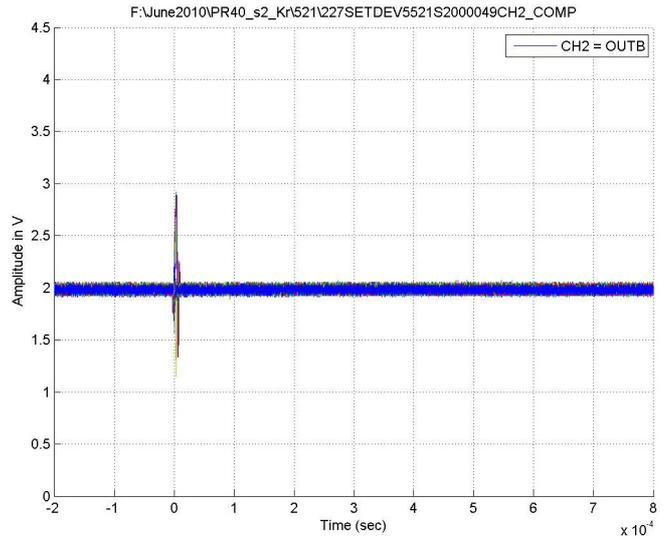
Figure 22. Typical Capture at  $V_S = \pm 4.5V$ , Channel B, LET = 28MeV·cm<sup>2</sup>/mg, Run 521
