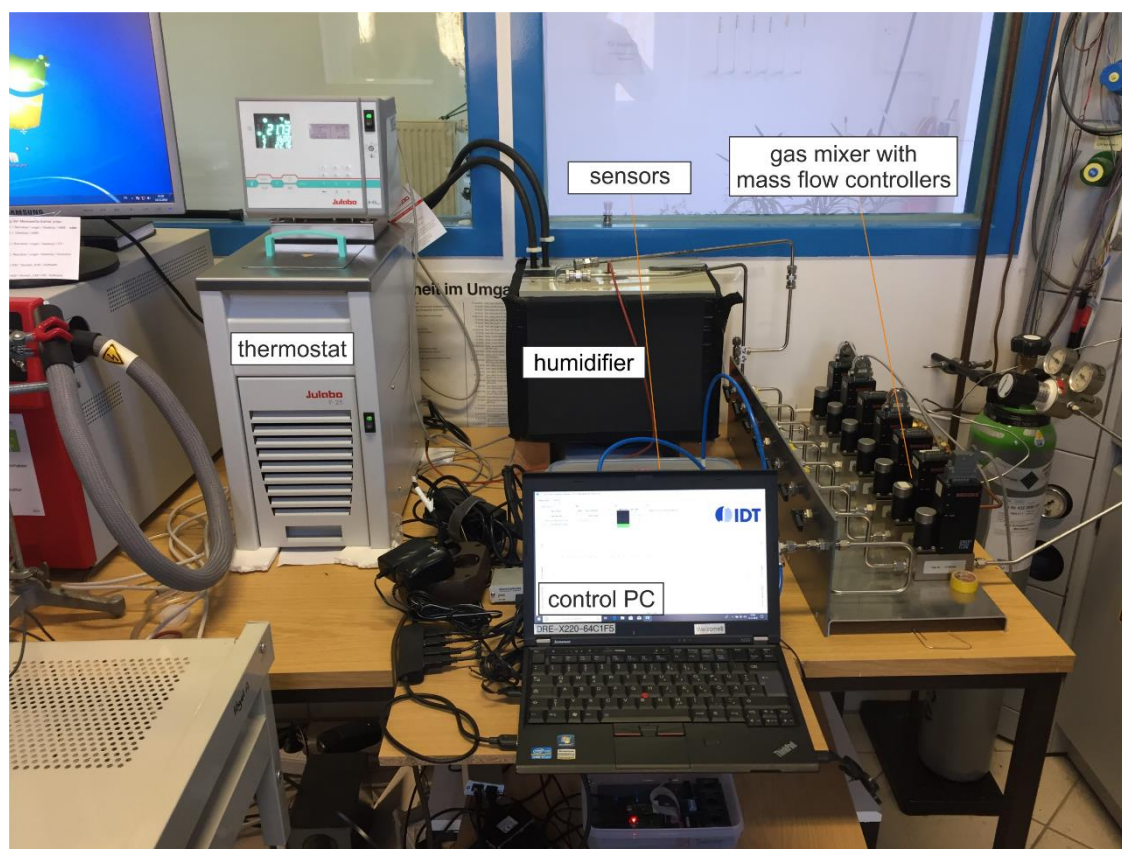
Fig. 2: Image of the calibration setup
