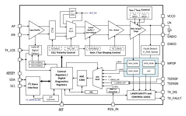
Figure 1: Functional Block Diagram of a single channel
