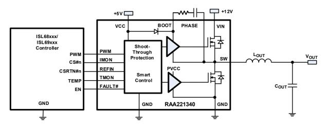
Figure 1. RAA221340 Simplified Application Block Diagram
