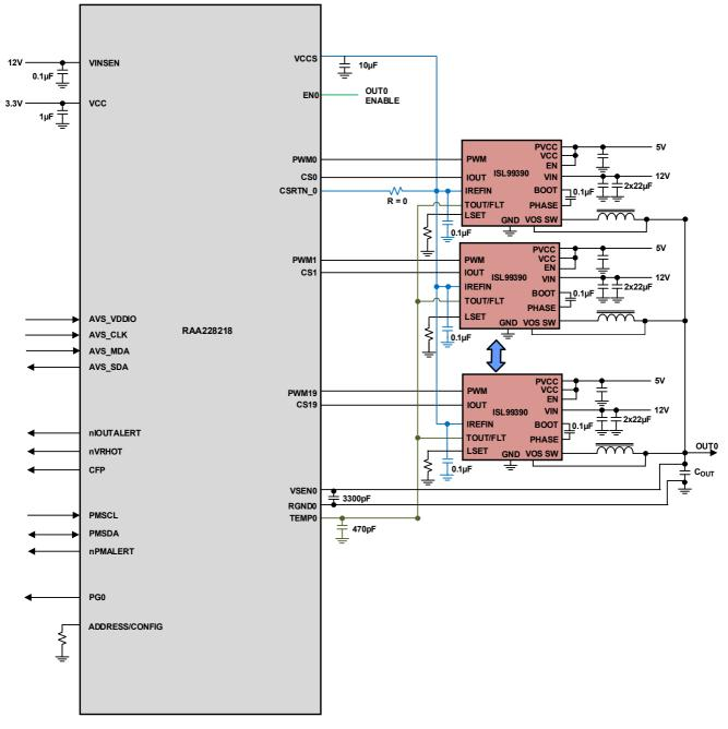
Figure 1. 20-Phase Smart Power Stage
