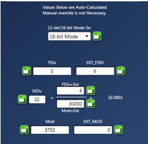
Figure 6. 8V97053 Feedback Divider Settings for 1.6 GHz + 5 kHz Output with 100 MHz PFD Frequency
